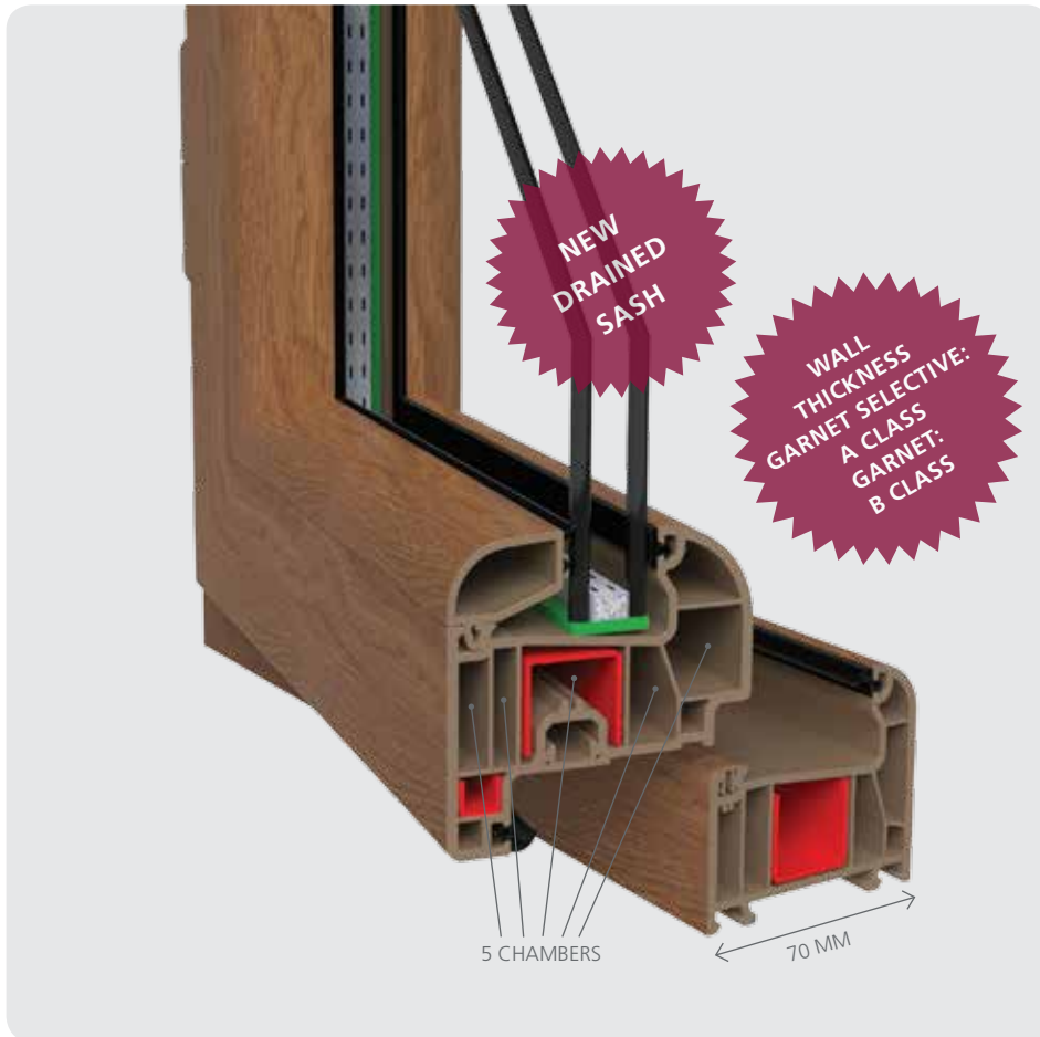
FRAME & SASH WIDTH 70 MM
